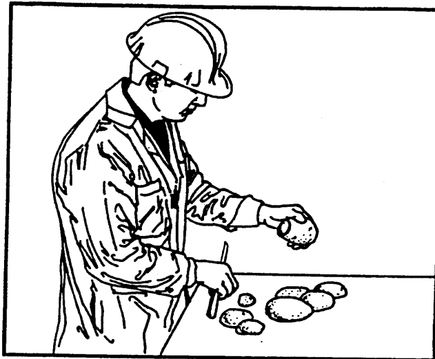
Figure 5-4. Cutting for internal examination.
