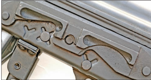
A side rail mount permits installation of all Eastern European scopes and night vision devices, including the 4x24mm and 6x42mm scopes available from Inter Ordnance.
