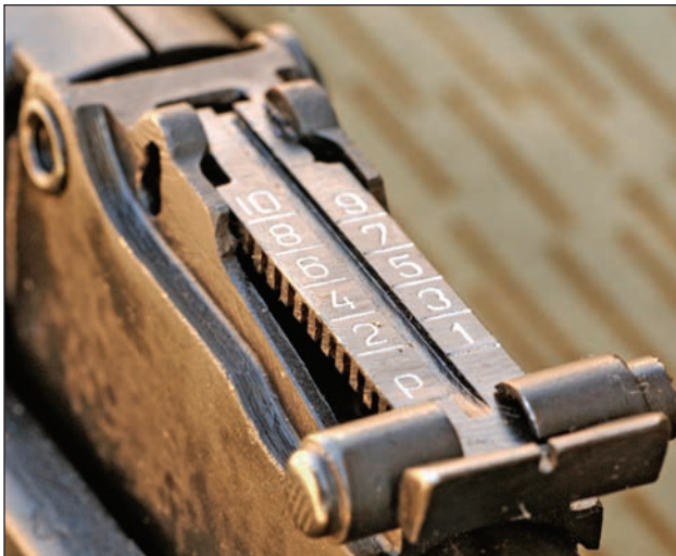
The rear sight is adjustable for elevation from 100 to 1000 meters. A battle sight setting, marked with a Cyrillic “P,” indicates ranges of zero to 300 meters.
