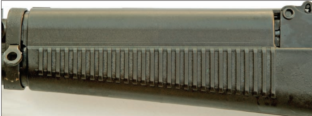
The two-piece forearm assembly tapers forward in a manner unlike that of any other AK. The eyelet on the locking pin serves as the front sling attachment point.
