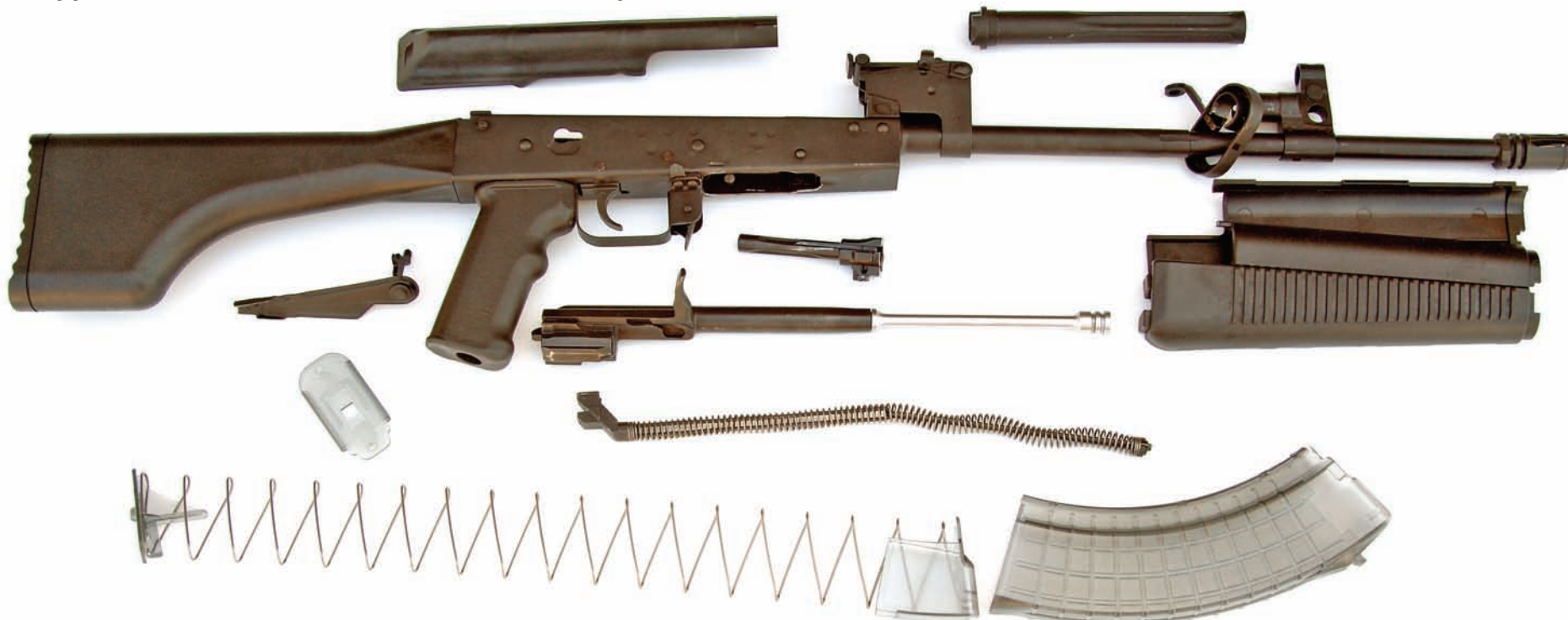
Except for the locking pin that retains the two-piece forearm assembly, disassembly procedures for the STG-2000-C are identical to those of any other AK.
