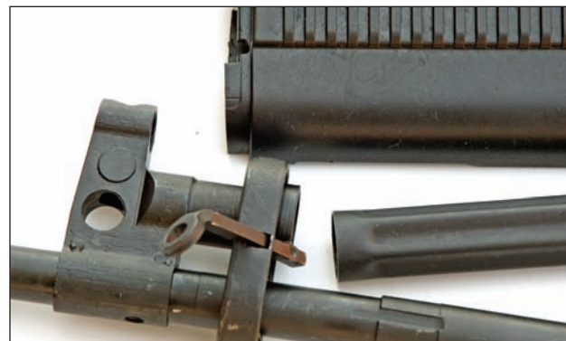
The sheet-metal cup that retains the two-piece forearm, as well as its captive lock pin and spring are proprietary and derived directly from the original Wieger 940.
