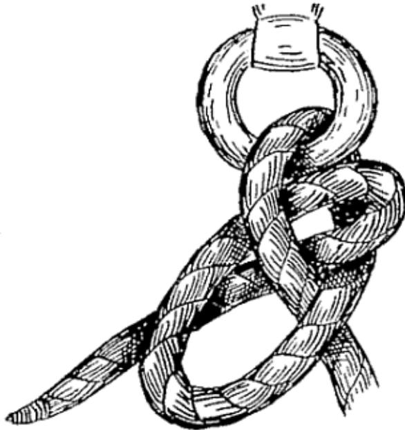
FIG. 33 —Slippery hitch (tying).
