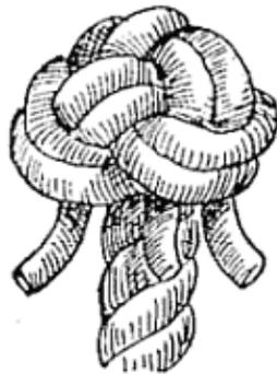
FIG. 126.—Double wall and crown.
