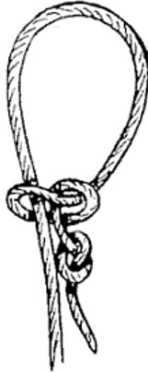
FIG. 65.—Loop knot.
