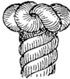
FIG. 114.—Wall knot.
