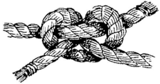
FIG. 14.—Slipped square knot.
