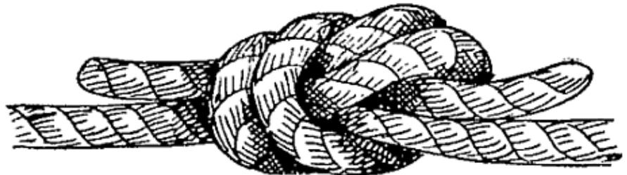
FIG. 19.—Ordinary knot (finished).
