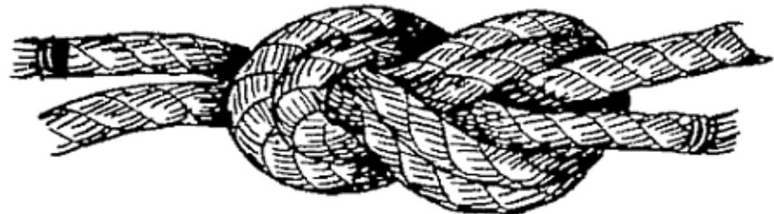
FIG. 24.—Double figure-eight knot (complete). is desired to prevent the rope running through an eye, ring, or tackle-block.
