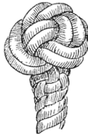
FIG. 127.—Double wall and crown (complete).
