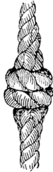
FIG. 117.—Shroud knot (complete).
