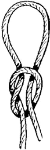
FIG. 62.—Loop knot.
