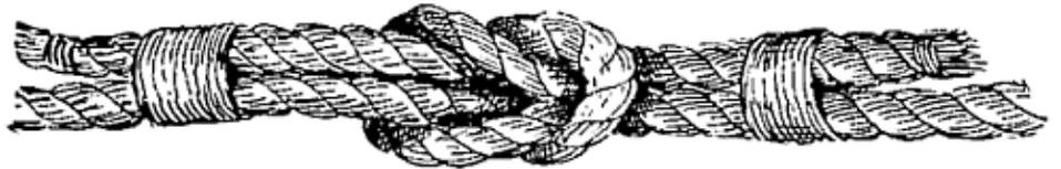
FIG. 15.—Square knot with ends seized.
