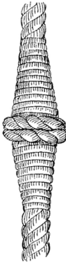
FIG. 120.—French shroud knot (complete).
