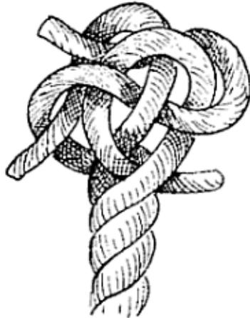
FIG. 121 A.—Making double crown.
