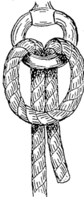
FIG. 31.—Lark's head with toggle (A) withdrawn.
