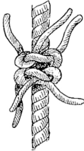
FIG. 118.—Shroud knot (making).
