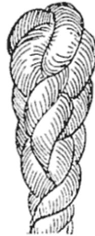
FIG. 113.—Single crown tucked (complete).
