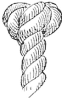
FIG. 122.—Double crown (complete).
