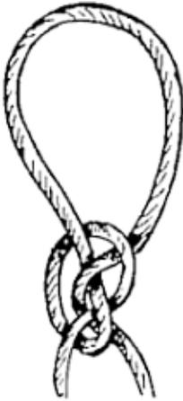
FIG. 64.—Loop knot.
