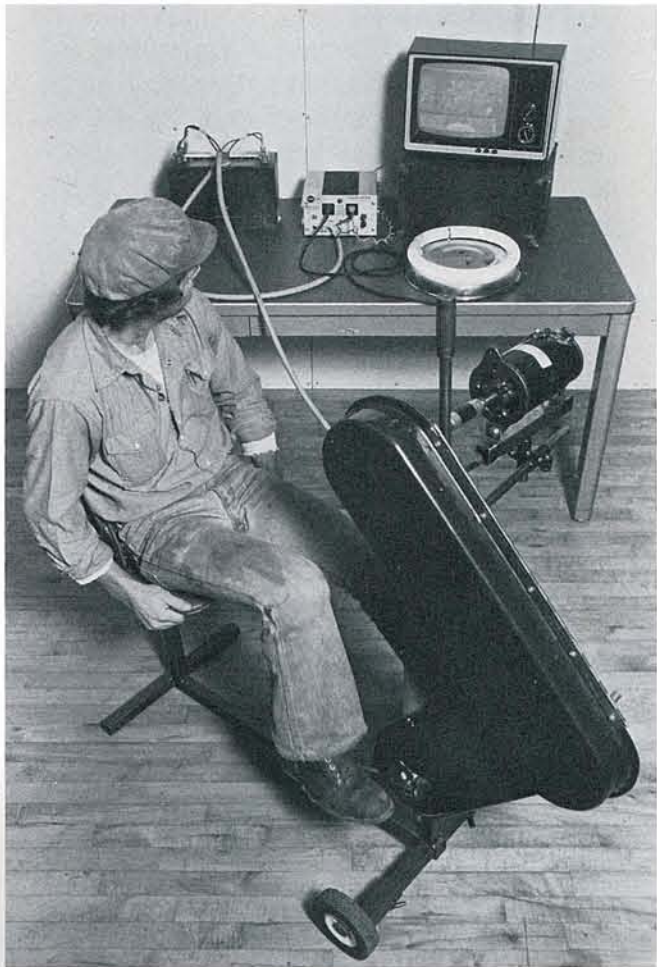
Figure 3-14 Generating electricity with the Energy Cycle
