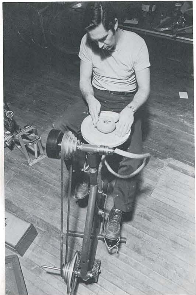
Figure 3-10 Potter's wheel powered by Energy Cycle
