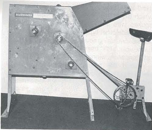
Figure 2-12 Commercial maize sheller (Courtesy of Ransomes Sims & Jefferies Ltd., Ipswich, England)
