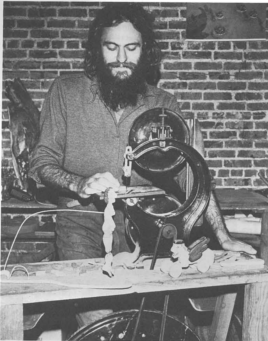
Figure 5-1 Treadle-driven machines allow for delicate workmanship.
