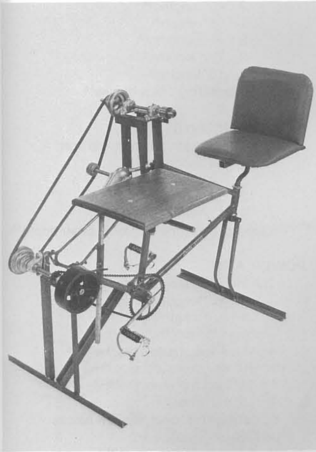
Figure 3-32 Homemade Energy Cycle built by Rodale R & D for less than $60
