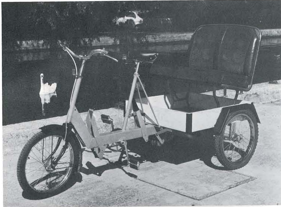
Figure 2-8 Oxtrike with temporary seat
