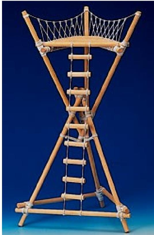
Six-Pole Towers: Here is a six-pole tower design, that uses two tripods. Stacking tripods like this results in a tower that is taller than the longest support poles. The lower tripod should always be larger and wider than the upper one, or weighted with anchor logs or stones, for structural stability.
