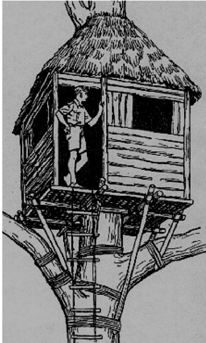
Treehouse Tower: any sturdy tree can be made into a tower, by building a platform on top, and making a ladder to reach the platform. The platform can be open, roofed, or fully enclosed, and the tree can be left whole, or the top can be removed (before constructing the platform). Existing branches can be used as supports, and extra supports can be lashed to the tree, as shown here.
