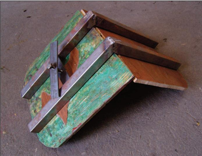
The seat is recycled plywood. The support is made from thin box section steel. See construction drawings for more detail.
