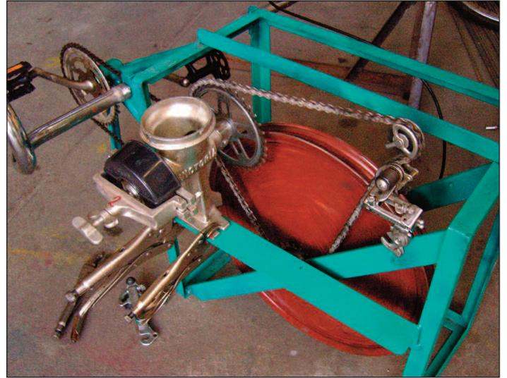
Now you can add a gear shifter. A simple friction type is best than an index shifter. Use the adjustment screws on the derailleur to make sure it selects all gears without the chain coming off.
