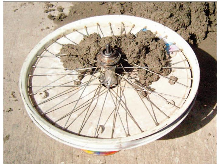
Mix the cement with two parts sand. Place the wheels on a bucket to provide support.
