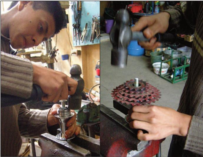
The Flywheel is made from a 20" wheel. Both ends of the hub must be threaded to accept sprockets. This can be achieved either by cutting and welding the threaded end from another hub, or by replacing one side of the hub and rebuilding the wheel. The welding option is easier but prone to causing undesirable wobble in the cassette.
