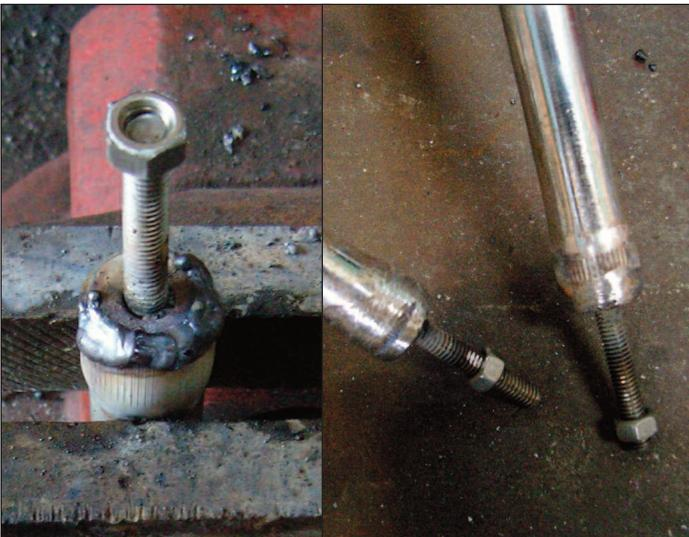
These are then welded onto to cut ends of the handlebar and filed smooth. They are then ready to be bolted onto the chassis.
