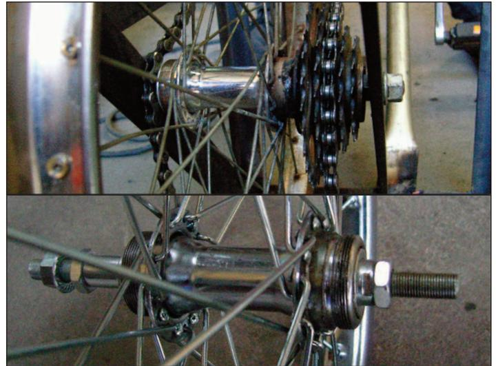
This split image shows the two options. Above is welded, below is a rebuilt hub. The hub is a push fit construction so it's possible to prise off the redundant unthreaded piece, and tap on a threaded one from an identical hub. Fit spokes using a screwdriver, rather than a spoke tensioner for speed.
