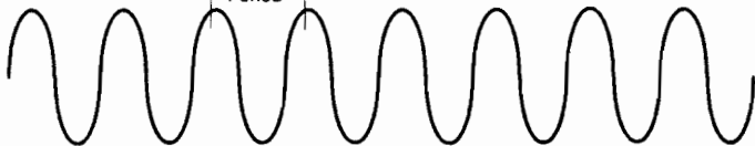
A. Unmodulated RF carrier wave
