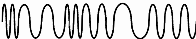
C. Frequency modulated (FM) RF carrier wave
