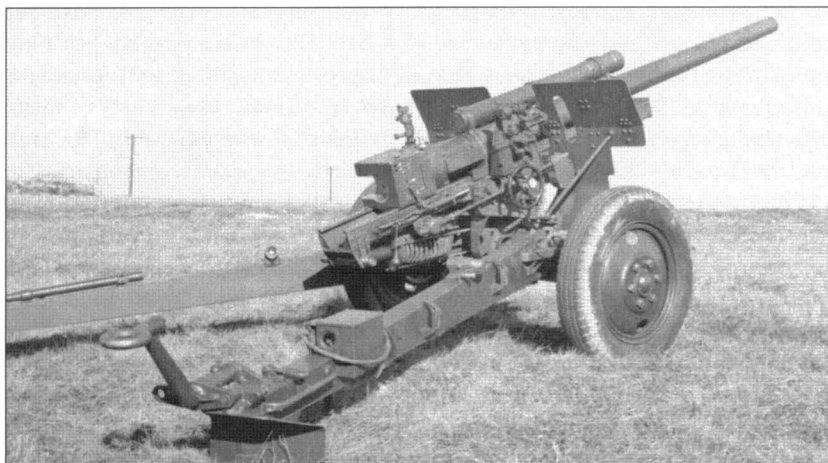
The 3in anti-tank gun was developed by mating a 3in anti-aircraft gun tube to the carriage and recoil mechanism of the new 105mm howitzer. Here the pilot 3in T10 gun on T1 carriage is shown during trials at APG in November 1941. (USAOM)
