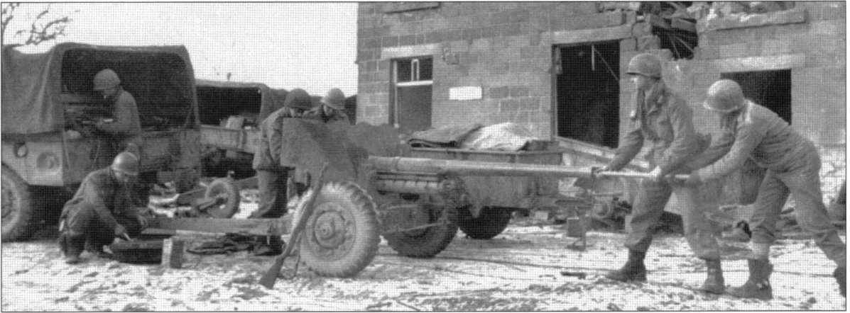
The final version of the 57mm gun to enter service included the M2 carriage, distinguishable by a caster wheel on the right trail to assist in moving the gun. Here it can be seen folded upward in the travel position. This gun crew from the 334th Infantry, 84th Division is servicing their gun in Marche, Belgium on January 2, 1945 during the Battle of the Bulge. (NARA)
