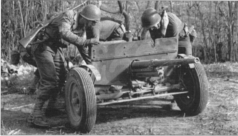
The first large-scale use of the 37mm anti-tank gun was in Tunisia in 1942–43. By the time it entered combat against the Wehrmacht, German panzers had been improved to the point where their frontal armor was largely impervious to the 37mm gun. (NARA)
