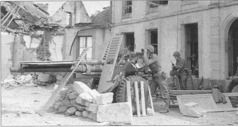
A camouflaged 3in gun in its defensive position during the fighting in northern France on August 19, 1944. The inadequate performance of the 3in gun against the German Panther, as well as its lack of mobility, led the US commanders in Europe to insist that it be replaced by a 90mm gun as soon as possible. (NARA)
