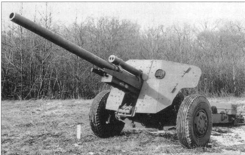
The 90mm anti-tank gun arrived too late to see any extensive use in World War II. A single example was sent to Germany in February 1945 as part of the Zebra mission, but saw little if any combat. When standardized, it was designated as the 90mm M26 gun on M18 carriage. (NARA)
