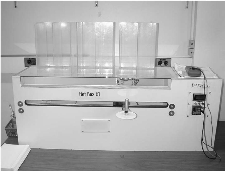
Fig. 2. A Hargreaves-type device prepared to permit concurrent testing of six rats. Note the presence of a Voltmeter on the instrument used for tracking changes in stimulus intensity over time.
