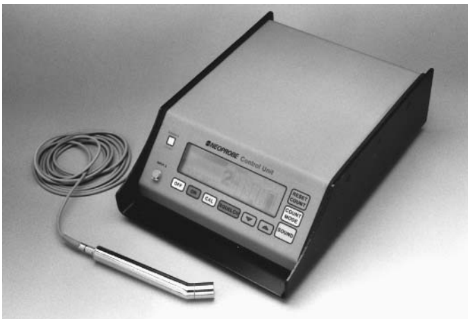
FIGURE 6 Hand-held gamma probe and control box (Neoprobe 1000, Neoprobe Corporation, Dublin, OH, U.S.A.).
