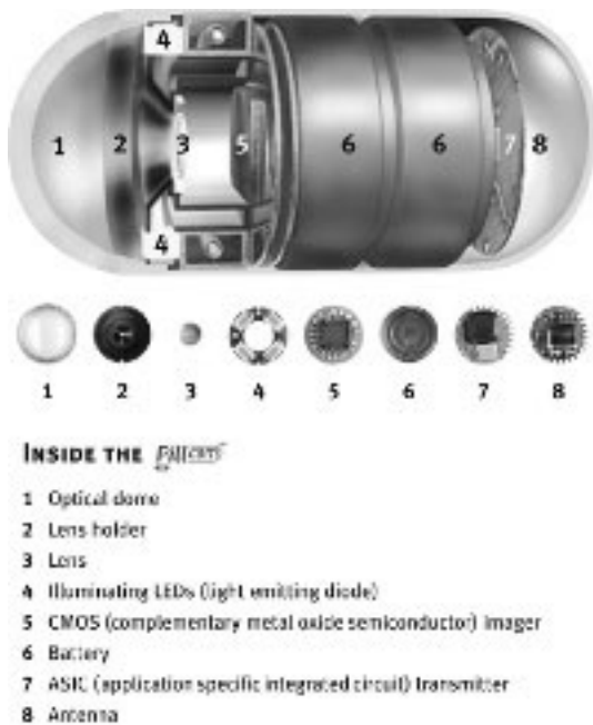
Fig 7.2 Inside the PillCam™ capsule endoscope.
