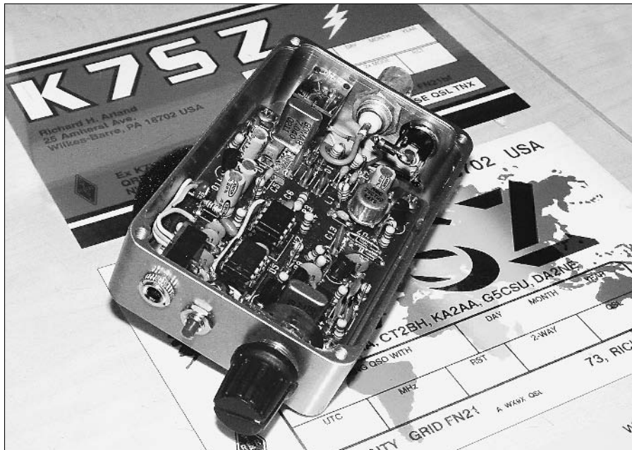
Figure 11-4: The RockMite transceiver fits in a mints tin!
